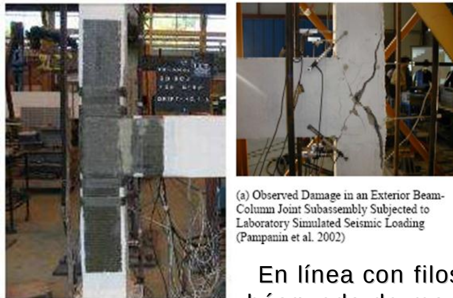
(b) Laboratory Retrofitted Unit (Akuzel and Pampanin 2007)
