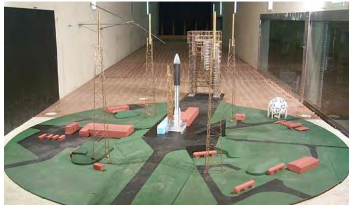
Figure 4: Aeroelastic model of the Atlas V Launch Vehicle with the Mobile Service Tower backed away to the rear.
