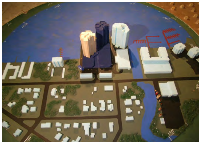
Figure 9: Thirty-storey Florida condominium, with tall proximate neighbours, used to compare balsawood force balance (shown here on the left as the twin building) data with the simultaneous pressure technique. The subject building is the middle one. Note that north is at the top of the photograph.
