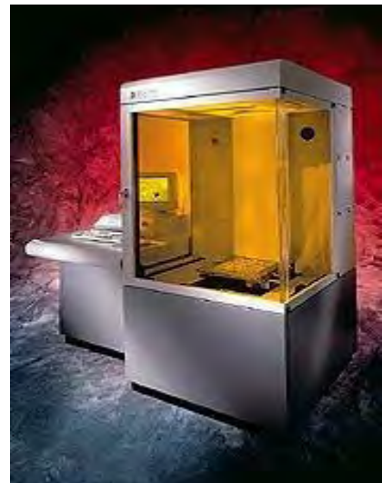
Figure 1: The laser booth and operational console of a stereolithography machine used to make complex wind-tunnel models with pressure taps included.
