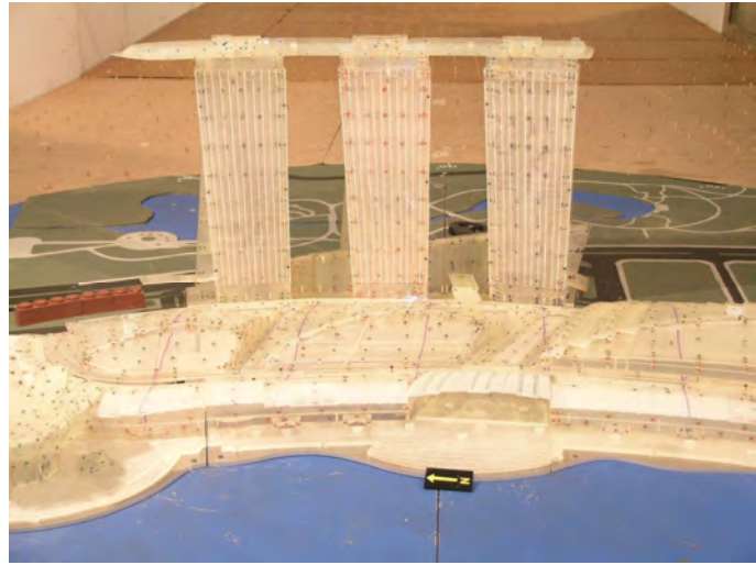
Figure 8: Over 3000 pressure taps were used to assess wind loads on key portions of the Marina Bay Sands development in Singapore - including the rooftop "bridge" garden on the three towers and some large lowrise canopies.
