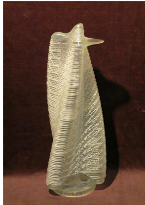
Figure 19: Al Raha Beach Tower, Abu Dhabi, makes good use of varying the building section over the height to decorrelate, or “confuse” the wind.
